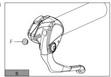
• Insert cable (G - Fig. 6) making it go through hole (H – Fig. 6) of the brake lever and the hole in fixing screw.
