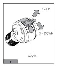
• By briefly pressing one of the two MODE buttons (Fig. 1 / 2) it is possible to view the battery charge level on the LED of the interface.
